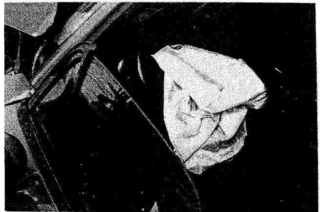
Picture 3: Driver seat of the case II with deployed airbag (see description in text).
