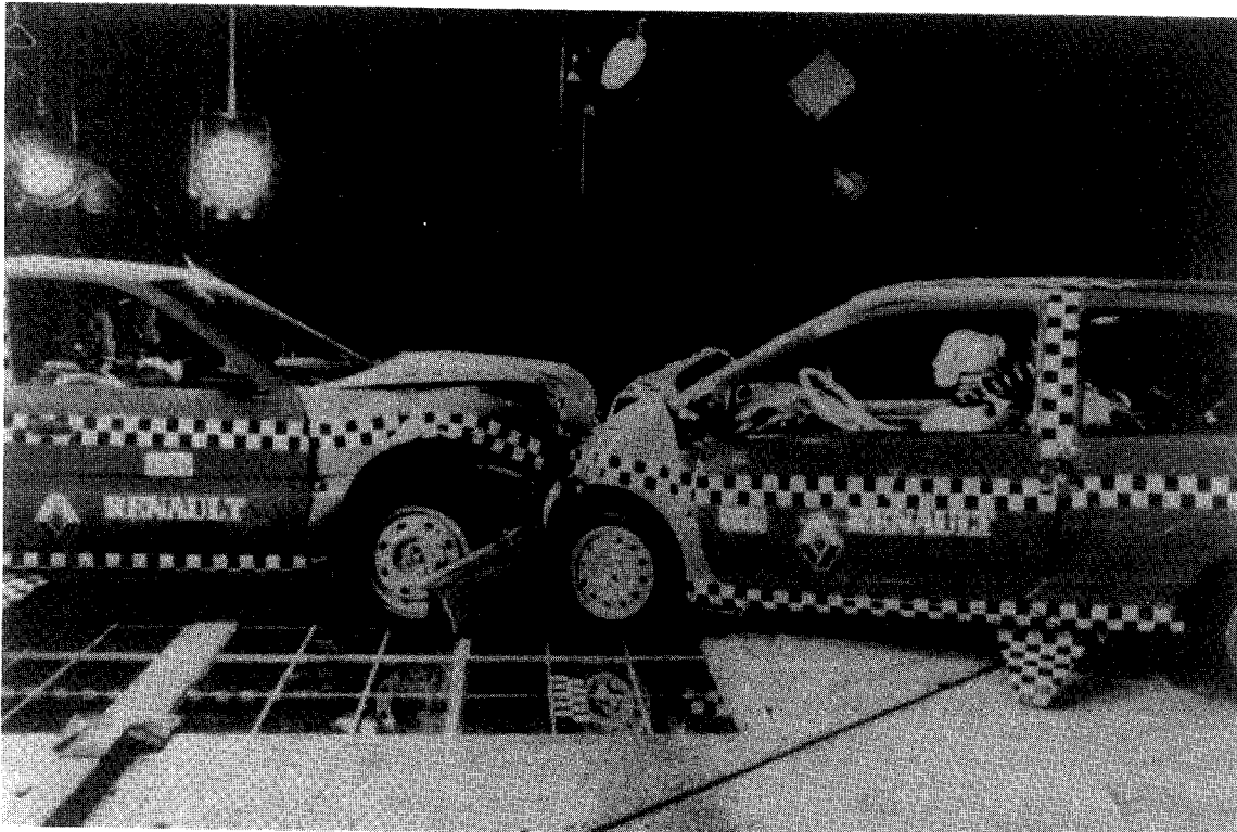
Head-on collision between a RENAULT Safrane and a RENAULT Twingo at closing speed of 80 km/h
